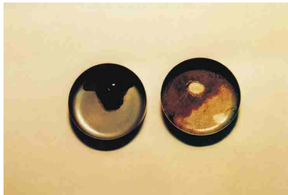
Fig. 5: Residues after storage at +250 °C, right: TURMOFLUID® 40 BK, left: an unfavourable competing oil
