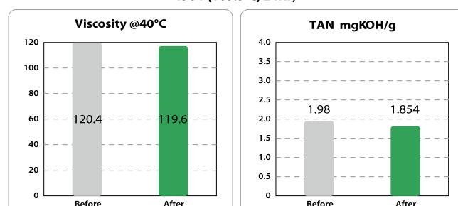
Oxidation stability test, ISOT, shows the viscosity of before test and after are almost the same.
